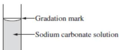
Step 4. The standard sodium carbonate solution in the pipette was transferred to the conical flask. The student ensured that all of the sodium carbonate solution was transferred to the conical flask by blowing through the pipette. Three drops of an appropriate indicator were added to the conical flask.
